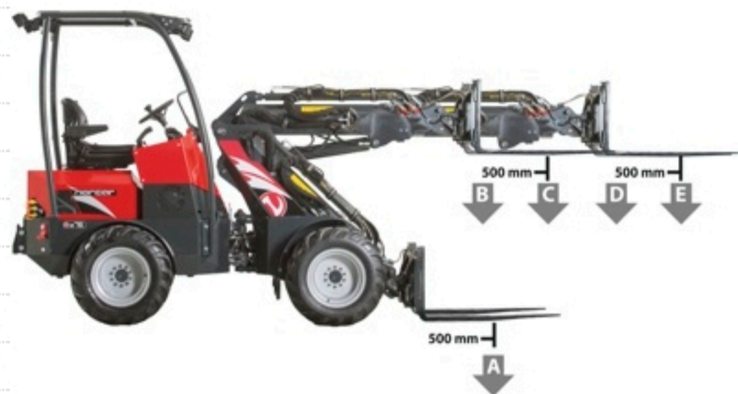
Standard machine +extra counter weights 270 kg
